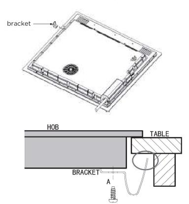
⚠ Under any circumstances, the brackets cannot touch with the inner surfaces of the worktop after installation (see picture).
