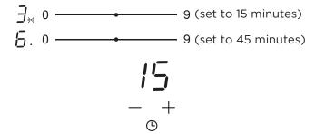
2. Once the countdown timer expires, the corresponding zone will switch off. Then it will show the new min. timer and the dot of corresponding zone will flash.
