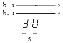
• Touch the heating zone selection control, the corresponding timer will be shown in the timer indicator.
