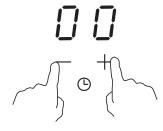
4. When the time is set, it will begin to count down immediately. The display will show the remaining time and the timer indicator flash for 5 seconds.
